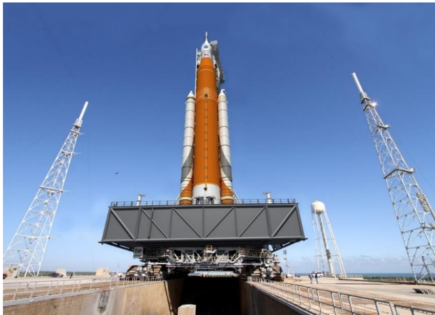
Figure 1. Artist Conception of the Space Launch System (SLS) and Mobile Launcher (ML) on the Crawler-Transporter (CT) (from http://www.nasa.gov )
