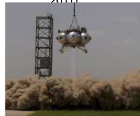
Regolith dust cloud formation during Morpheus lander plume impinging on Mars simulant (Morpheus, 2013)
