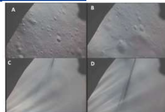
Apollo 15 LEM camera views showing progression of plume-regolith interaction resulting in high speed particle sheets obscuration. (Metzger, 2011)
