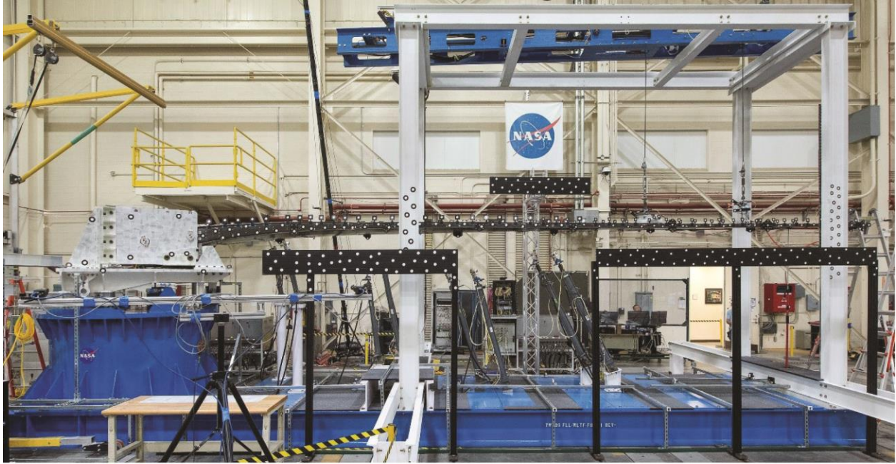
Figure 10. The test setup for the Passive Aeroelastic Tailored wing.
