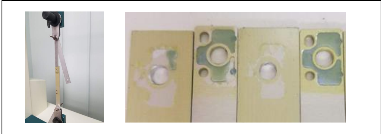
Figure 7 - Liquid Pin Joint Shear Load Measurement Test Setup and Coupons after Joint Failures
