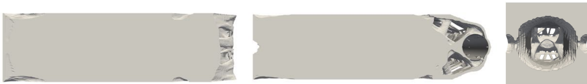
Figure 38: Top, side, and rear views of the stress- and frequency-constrained mass minimization result for the cantilever beam problem
