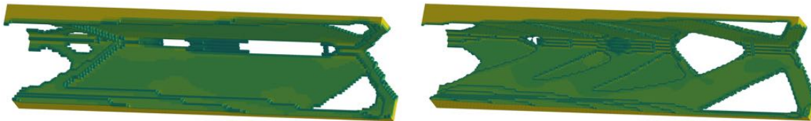
(a) Design obtained using 24 processors for mesh with 525,987 degrees of freedom.
