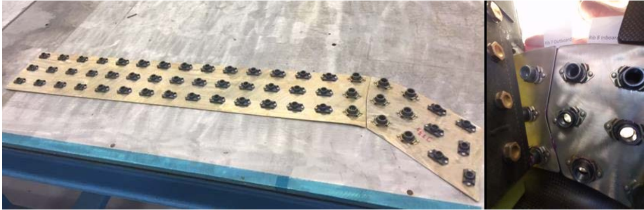
Figure 5.7. Nutplate carrier assembled (left) and installed (right).
