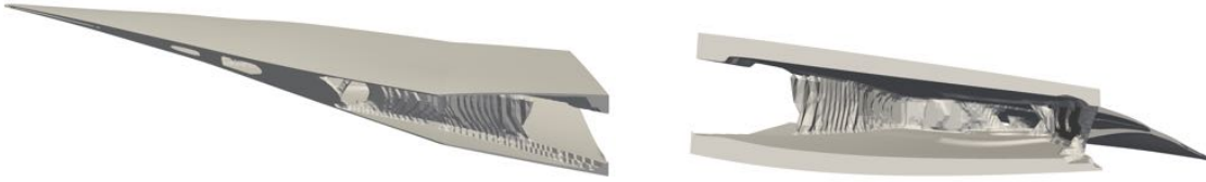
Figure 28: uCRM wingbox compliance minimization results. Leading edge (left), wing root (right).
