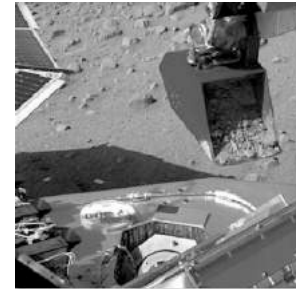
Fig 1: Mars Phoenix mission ISAD Scoop
