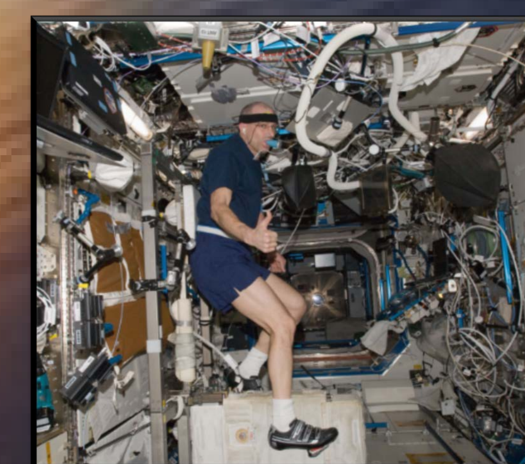
Figure 2. In-flight VO 2 pk test using the Portable Pulmonary Function System (PPFS) and CEVIS.
