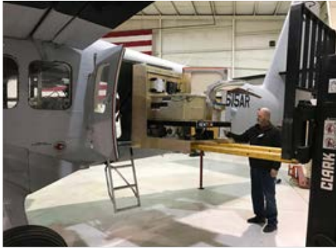
Figure 3. The SWESARR instrument during integration to the Twin Otter aircraft prior to the radar's first test flights.
