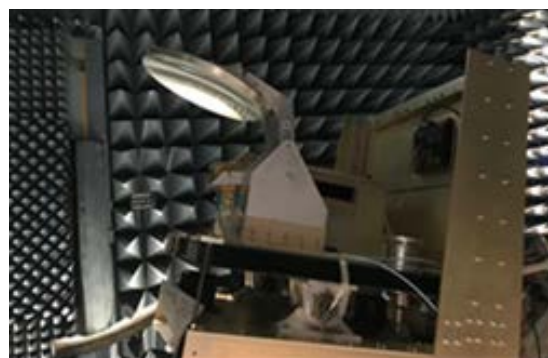
Figure 1. SWESARR, a tri-band radar and radiometer airborne system designed to retrieve snow water equivalent (SWE), during testing at NASA GSFC's anechoic chamber.
