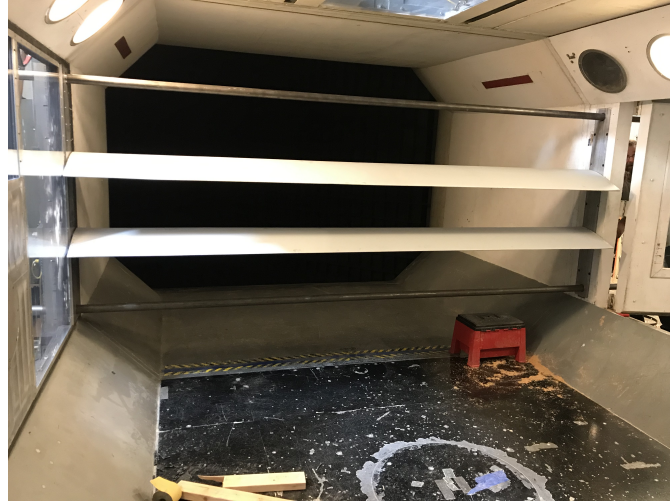
Fig. 4 UWAL gust generator installation
