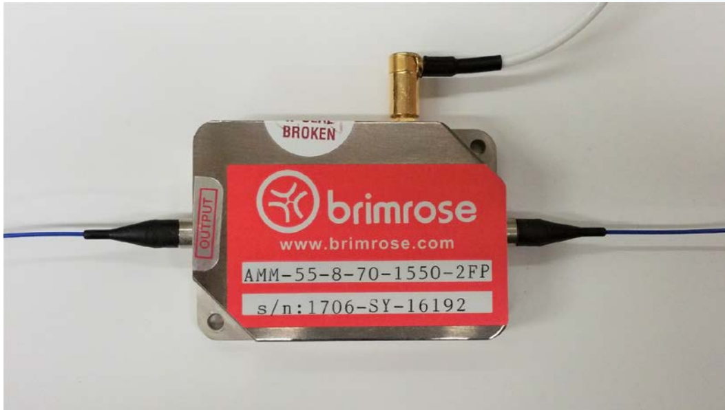
Acousto-Optic Modulator (AOM): 45 dB max extinction ratio, max frequency 55 MHz
