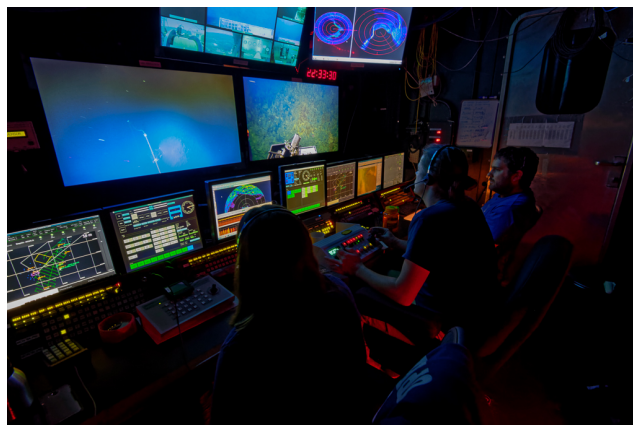
Figure 3. E/V Nautilus control van during ROV operations. Argus and Hercules pilots and navigator were seated at the monitors (foreground to background in image). Not pictured: Data logger, chief scientist and watch lead sat in second row (Photo Credit: OET).
