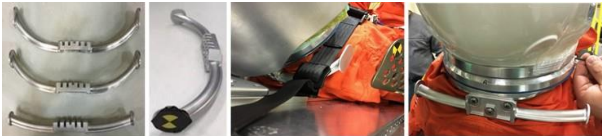
Figure 3. Rigid Countermeasure Prototypes and Installation
