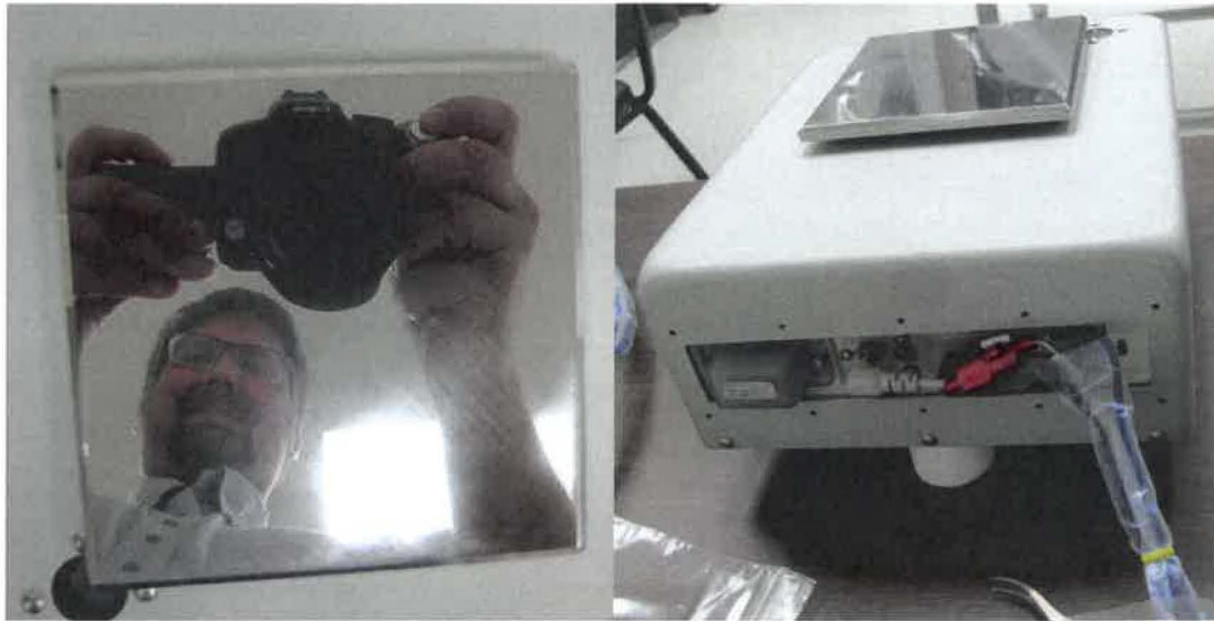
Fig. 7: Left image shows the custom 316L stainless steel weighing plate. Right image shows the back cut-out for the wire harness and Bluetooth. During operations, this is enclosed with the PTFE and Viton seals.
