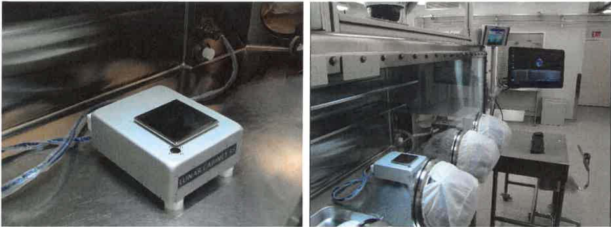
Fig. 5: Mettler-Toledo XP5003SDR balance custom housing, weighing pan, and wire harness integrated into the Lunar Processing Cabinet. The Right image shows the balance control screen and computer.
