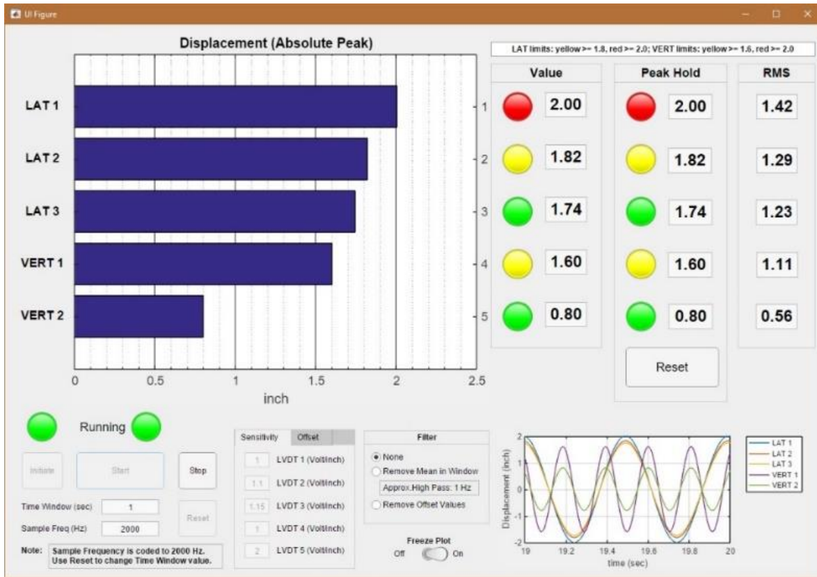
Figure 7: Hydraulic Shaker Displacement Monitor Interface
