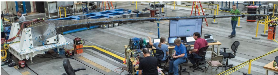
Figure 8: The simplified modal test setup: the Passive Aeroelastic Tailored Wing mounted on only the Wing Loads Test Fixture reaction table
