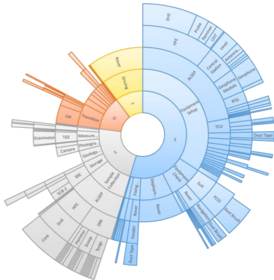
Fig. 1. EVA-1 Tasks for Commander Gene Cernan and Lunar Module Pilot Jack Schmitt.
