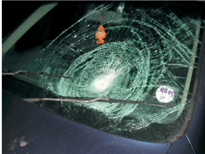
Figure 4.4: Example of evidence (pedestrian head contact damage to windscreen)
