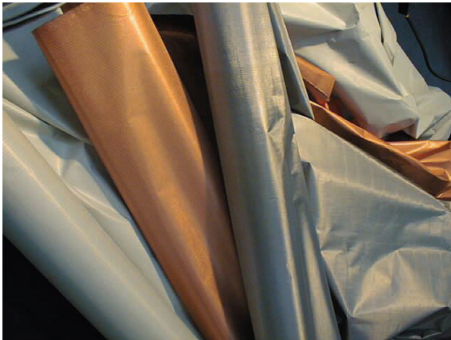
Figure 2-1 Conductive woven fabric from Shieldex (picture from [7])
