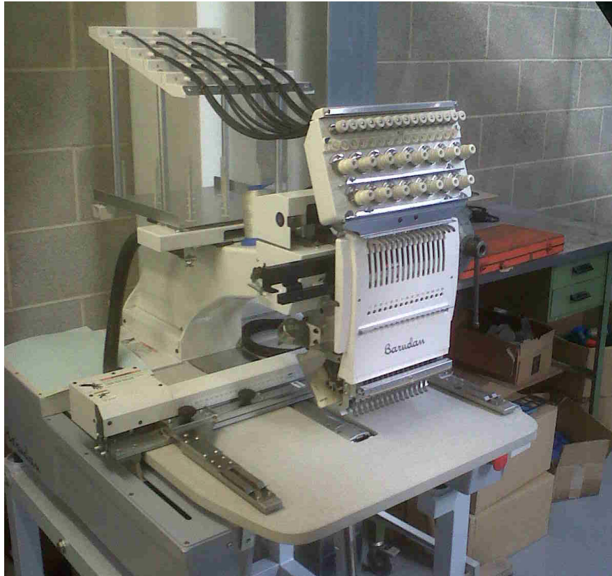
Figure 2-14 Computerised embroidery machine at Nottingham Trent University (model: Barudan BEVT-Z1501CB)
