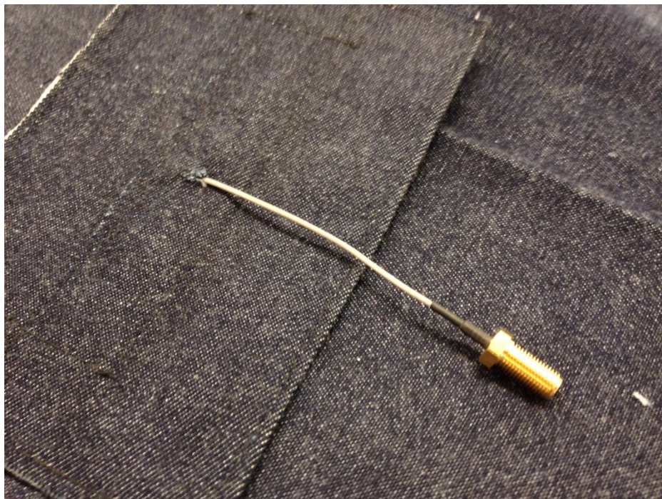
Figure 2-26 Covered low profile U.FL connector with flexible cable
