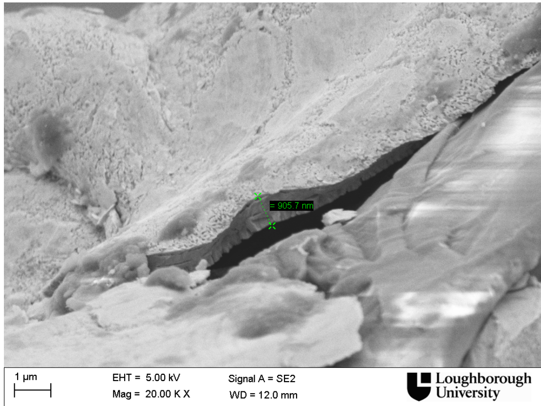
Figure 2-10 SEM image of broken section of coated layer
