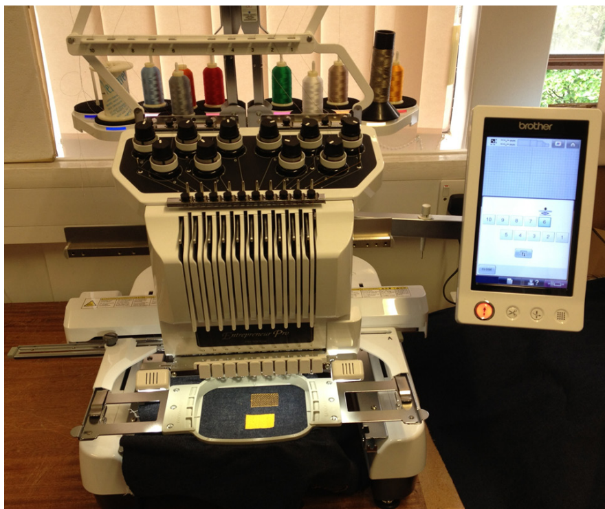
Figure 2-15 Computerised embroidery machine at Loughborough University (model: Brother Entrepreneur® Pro PR1000e)
