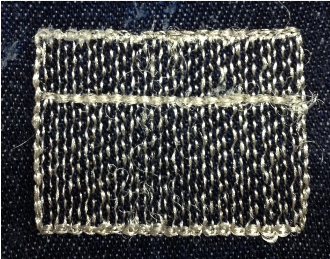
Figure 5-28 Embroidered 1 mm spaced non-uniform meshed patch on denim fabric
