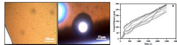
Non-aerated and aerated 50% coffee (B) frontal distance vs time plot of aerated 50% coffee freeze dried under FDM
