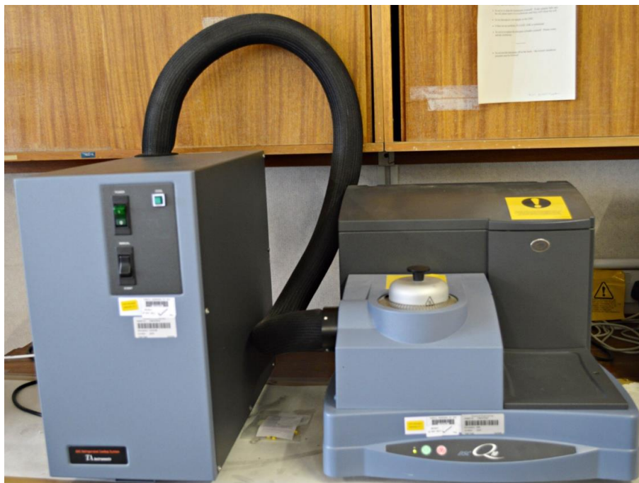
Figure 3.16: The TA Q10 DSC instrument used in this research
