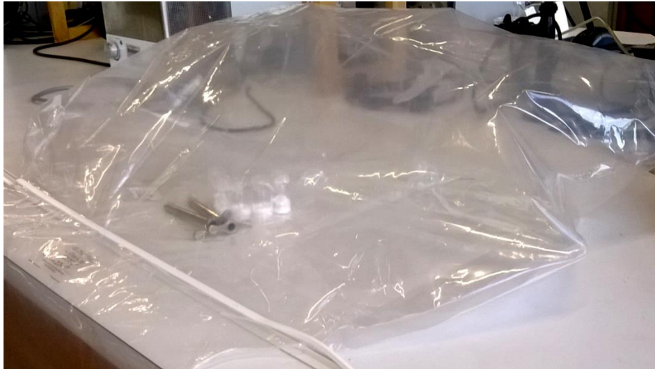
Figure B.1: Nitrogen purged glove bag used for storage of samples after freeze drying to prepare samples for FEGSEM to avoid contact with air.
