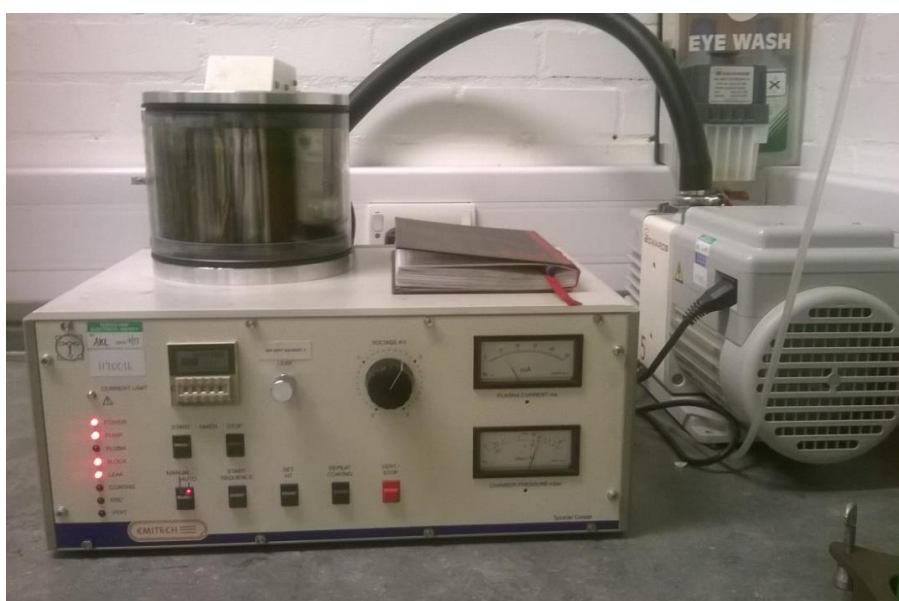
Figure 3.15: Gold/Palladium (Au/Pd) sputter coater used for gold coating of freeze dried samples before conducting FEGSEM
