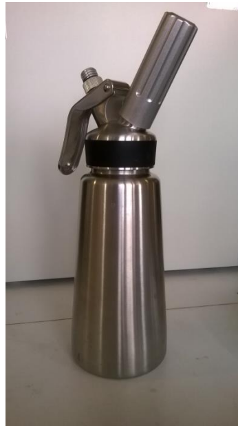
Figure 3.1: Cream whipper used for aeration of 50% coffee extract before freeze drying.
