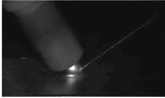
Figure d: Weld area capturing using HS camera, band-pass filter and laser illumination
