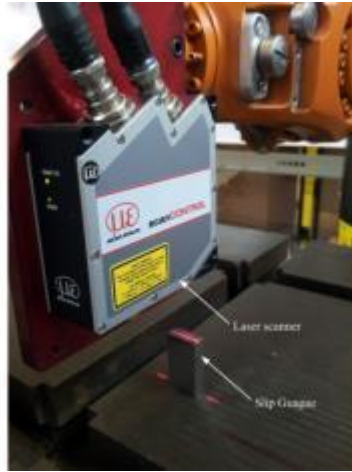
Figure 5-5: Setup for vertical resolution measurement
