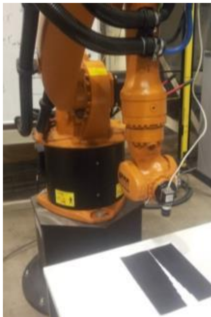
Figure 7-7: Setup for checking gap sensing performance
