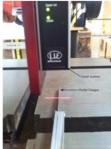
Figure 5-7: Setup measuring a metric feeler gauge and percentage error in measurements
