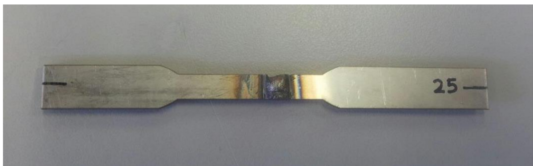
Figure 8-6: Specimen preparation for tensile testing
