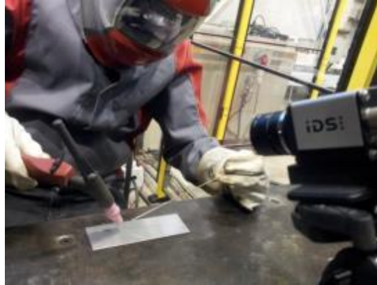
Figure 4-4: An image of the camera setup for testing a welder
