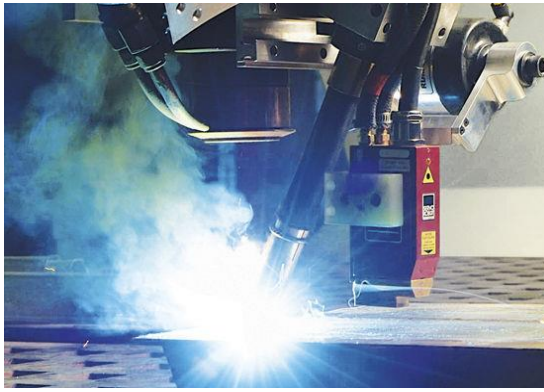
Figure 2-10: Laser scanner inspecting prior to welding[83]
