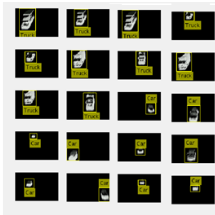
Figure 6.7: Classified vehicles using CENTROG feature descriptor
