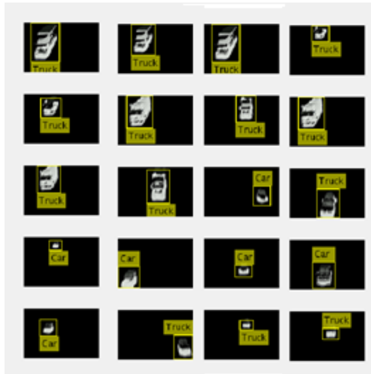
Figure 6.8: Classified vehicles using CENTRIST feature descriptor
