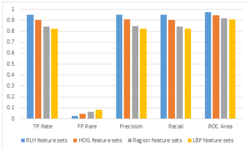
Figure 5.9: Weighted average plot of TP, FP rates, precision, recall and ROC area for RLH, HOG, Region and LBP feature sets
