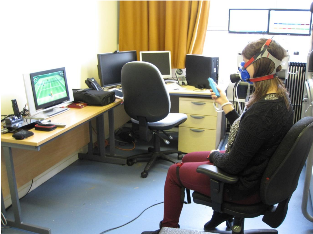
Figure 3.5 A picture of a participant undertaking the playing Wii condition and wore a face-mask, connected to an open circuit breath-by-breath automated gas-analysis system which measures expired respiratory gas fractions (Cortex Metalyzer, Leipzig, Germany) and provides an estimate of energy expenditure.
