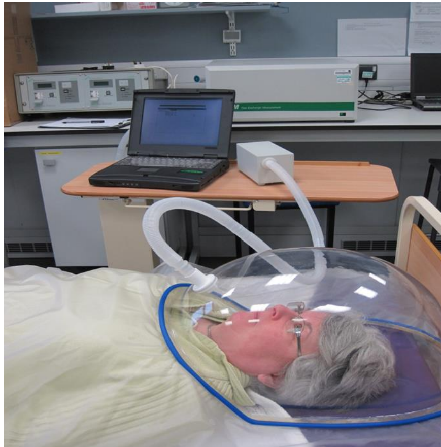
Figure 3.3. The measurement of resting metabolic rate using the GEM ventilated hood. The study participant is spending 60 minutes in a semi-supine resting position under the ventilated hood (GE Nutrition. UK).
