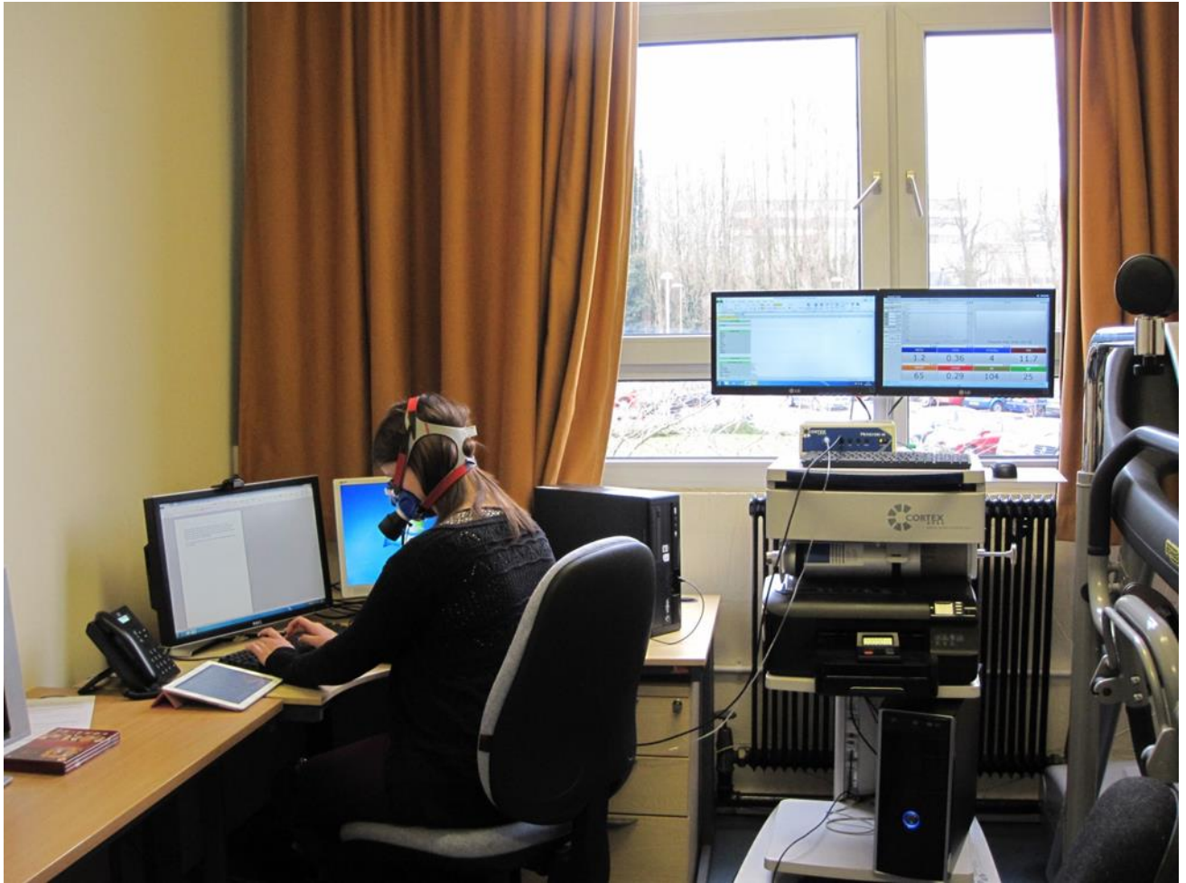
Figure 3.4. A picture of a participant undertaking the typing condition. The participant is wearing a face-mask, connected to an open circuit breath-by-breath automated gas-analysis system which measures expired respiratory gas fractions (Cortex Metalyzer, Leipzig, Germany) and provides an estimate of energy expenditure.
