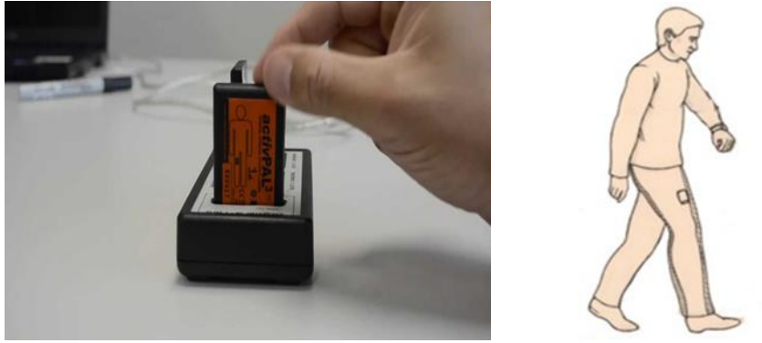
Figure 5.1. This figure shows the ActivPAL3 which participant wore on the anterior aspect of their thigh. http://www.paltech.plus.com/products.htm
