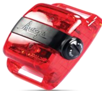
Figure 4.1. The ActiGraph GT3X+ (Actigraph LLC, Pensacola, FL, USA) is a small (4.6cm x 3.3cm x 1.5cm), lightweight (19g) tri-axial accelerometer. In this study participants wear one of the devices on their non- dominant thigh and another one around their waist
