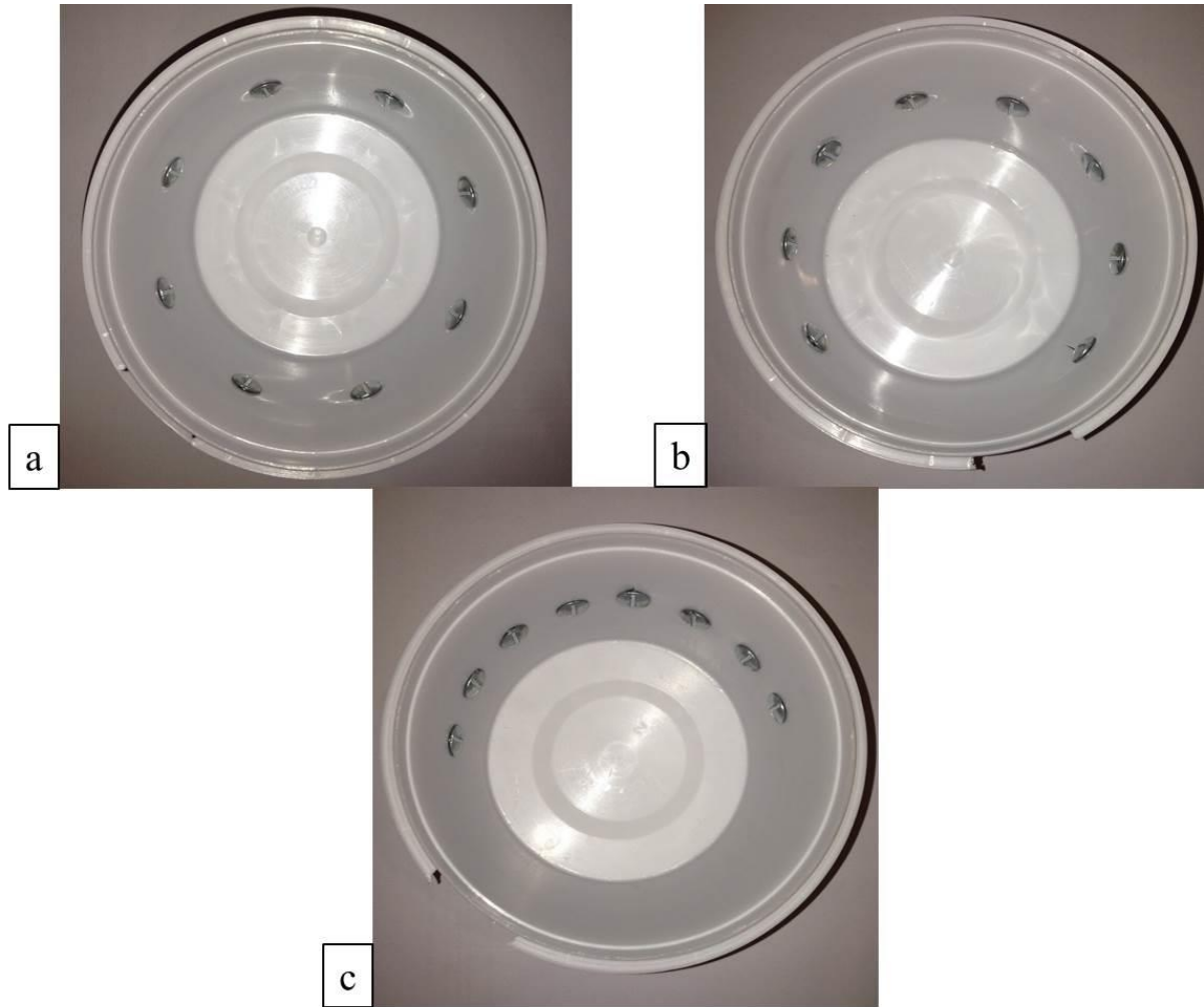
Figure 5-2: Phantom models showing (a) FA, the standard ring layout where the eight electrodes were placed equally spaced around the head. (b) SA, a novel electrode configuration applied to the front of the head separated by angle of 36^\circ in a semi-circular profile. (c) HA, an electrode configuration placed in a semi-circular profile by angle of 22.5^\circ . Screws show the electrode positions.
