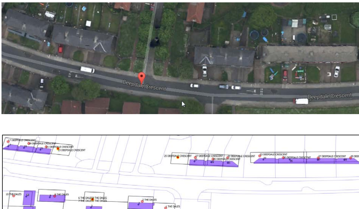
Figure 7-16 Use of Google Earth™ and QGIS™ to visually cross check roof and building data
