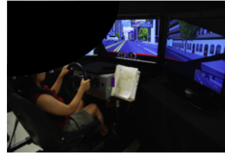
Fig. 1. The STISIM Drive™ M400 driving simulator in the Ergonomics Lab at NC State University.
