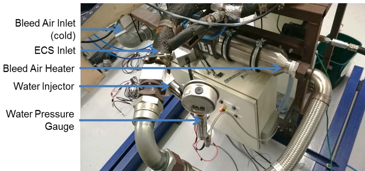
Figure 4-3: Bleed air supply emulators subsystem.
