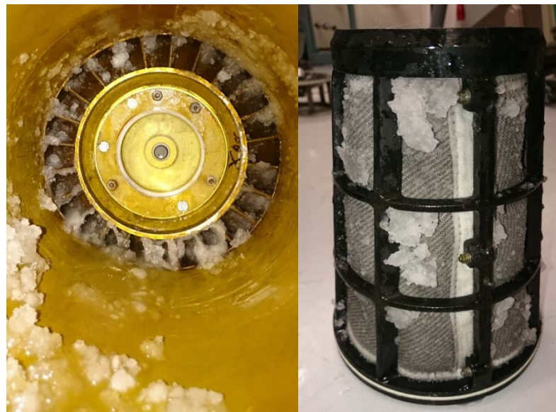
Figure 5-17. Water Extractor after Transient Icing Test. (a) shows the interior of WE, (b) shows the outside of the coalescing fabric element.
