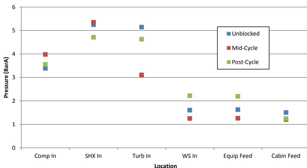
Figure 5-18: Cycle Blockage Comparison of component pressures.
