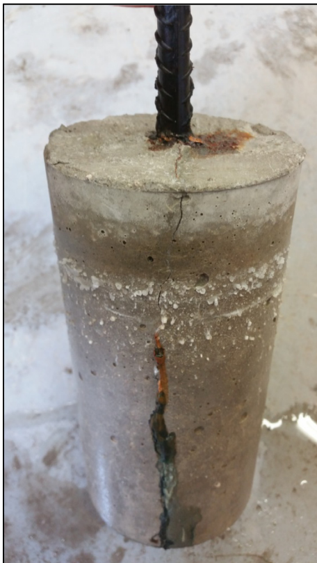
Fig. 3. Typical cracking of 200 mm × 100 mm diameter reinforced concrete cylinder.
