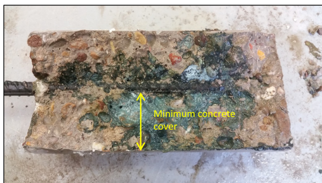
Fig. 4. Measurement of cover depth and development of 'green rust' precipitate.
