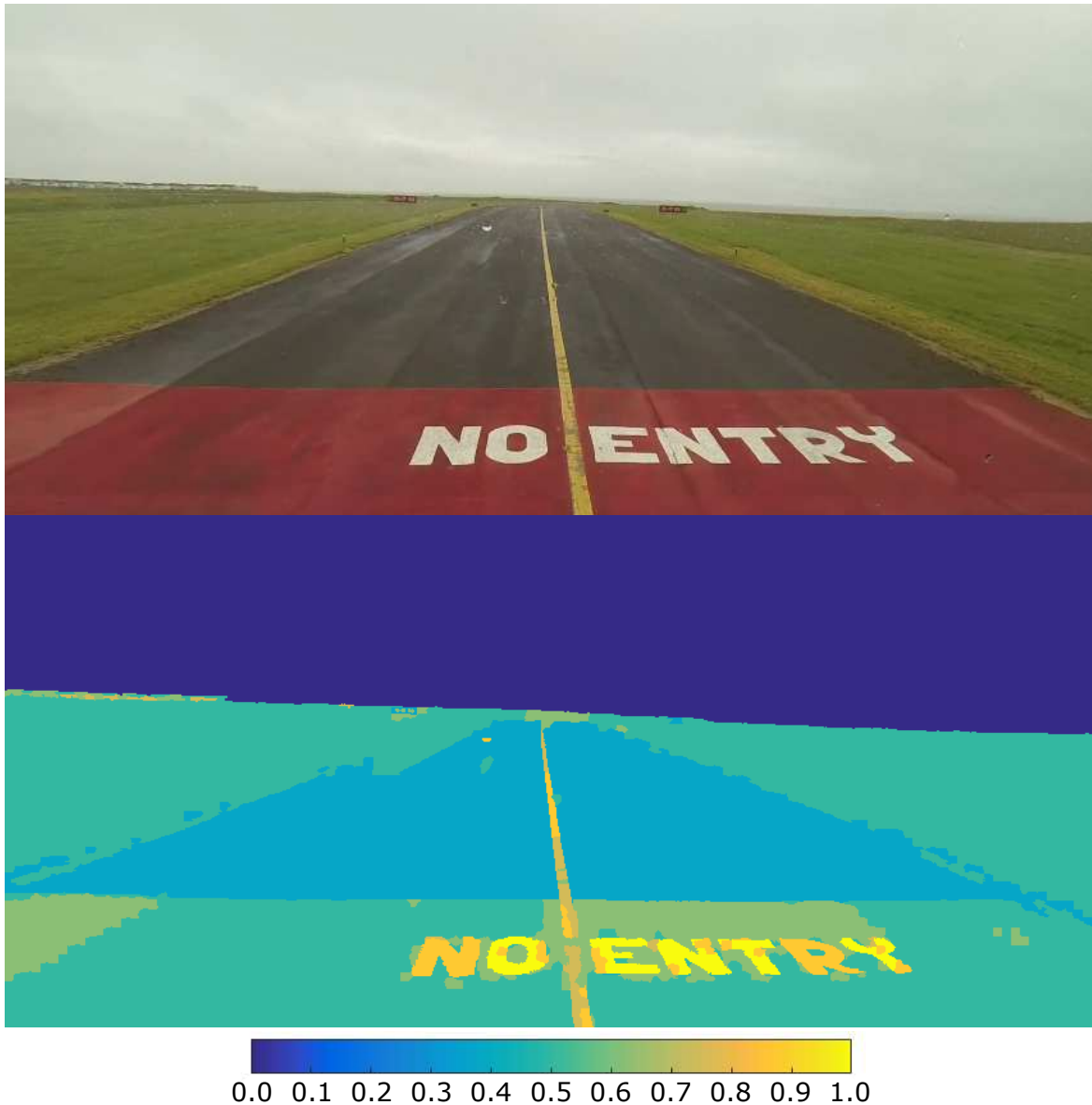
Fig. 6.31 Example of Normalised Relative Luminance, based on the original top image. It should be observed that despite being the brightest object in the original image, the sky region has been reduced to lowest likelihood of being classified as surface markings through the use of horizon detection. Instead, the surface markings within the image receive the highest NRL values, as intended. A more detailed evaluation of NRL imagery occurs in Chapter 8.
