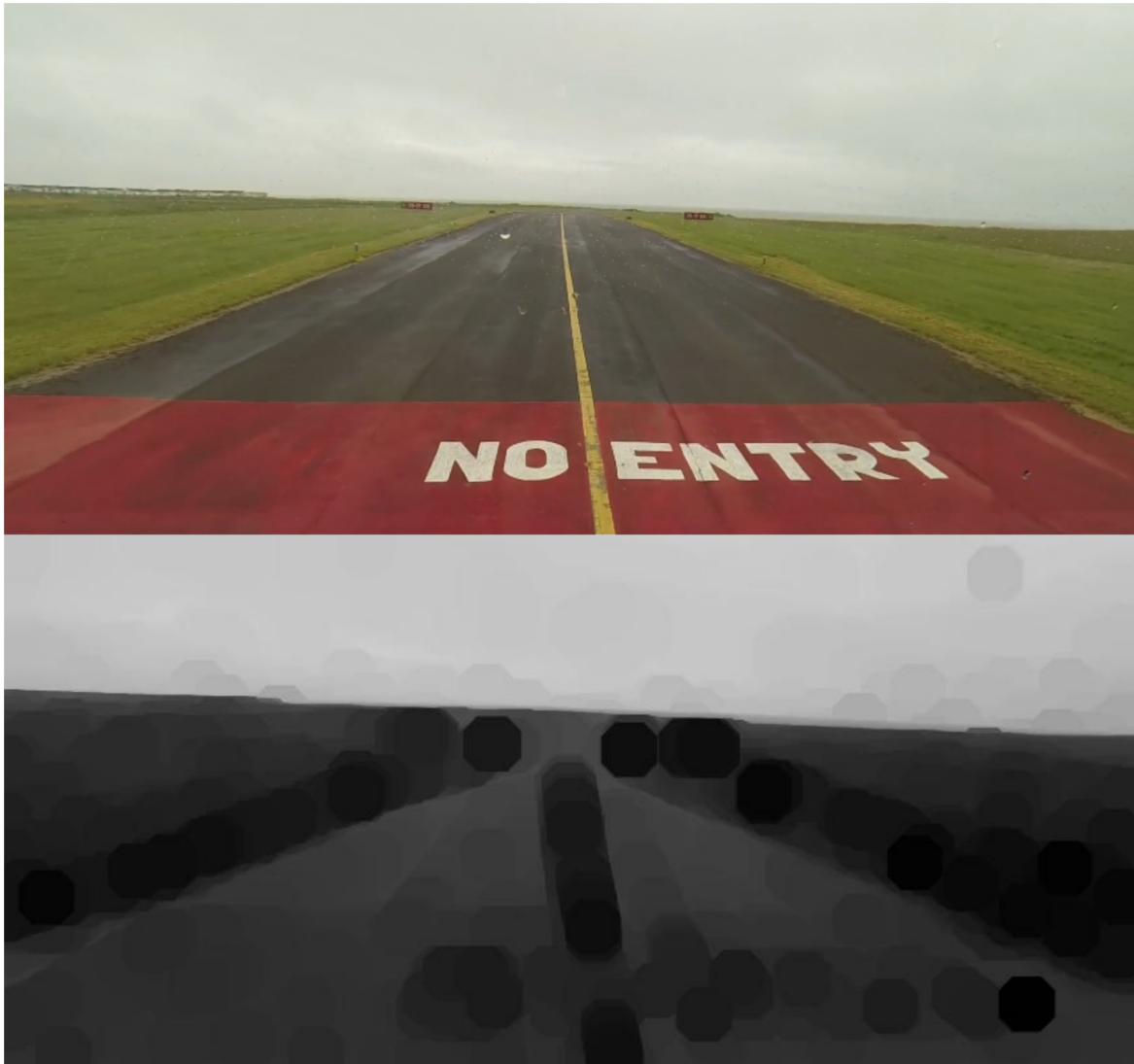
Fig. 6.32 Example of Dark Channel Extraction, based on the original top image. The distinct difference between sky and ground pixels allows the horizon line to be easily determined.
