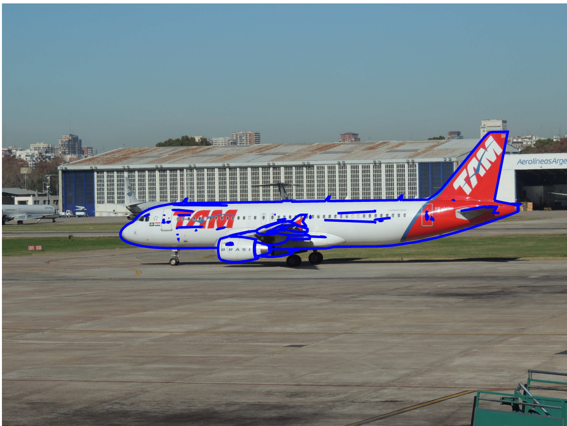
Fig. 4.4 Example of 3D shape based matching, using previous A320 model to detect real-world example. From the known camera parameters, the pose and orientation of the aircraft can be determined with respect to the camera. Object detection achieved here using MVTec Halcon.
