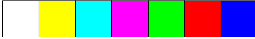
Fig. 6.28 Example of colours which share the same Value within HSV colour space, (the three colour primaries and white), indicating how Value is visibly separate from the human interpretation of brightness.
