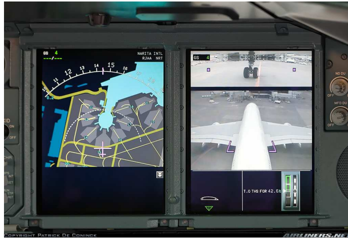
Fig. 2.1 A380 cockpit displays, showing OANS (left) and ETACS (right). ©Patrick De Coninck.
