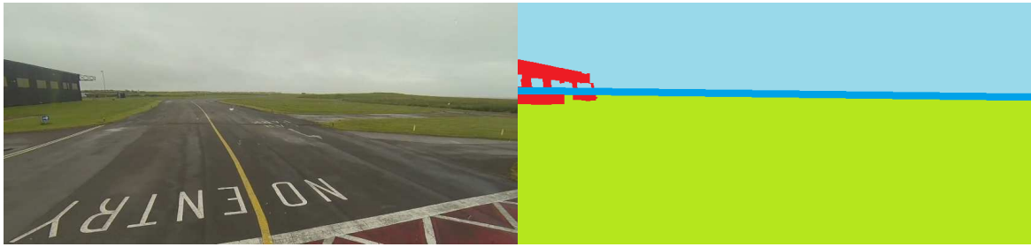
Fig. 6.34 Horizon based cluster classification. In the original image to the left, the only object which extends to each side of the horizon line is the building. This result is clearly reflected the horizon based classification on the right, where only the building cluster has been assigned the Intercept class. Although the windows in the building are not classified as intercept, as collision avoidance should always estimate to the bottom of objects, this collision risk has been potentially detection through horizon line extraction alone.
