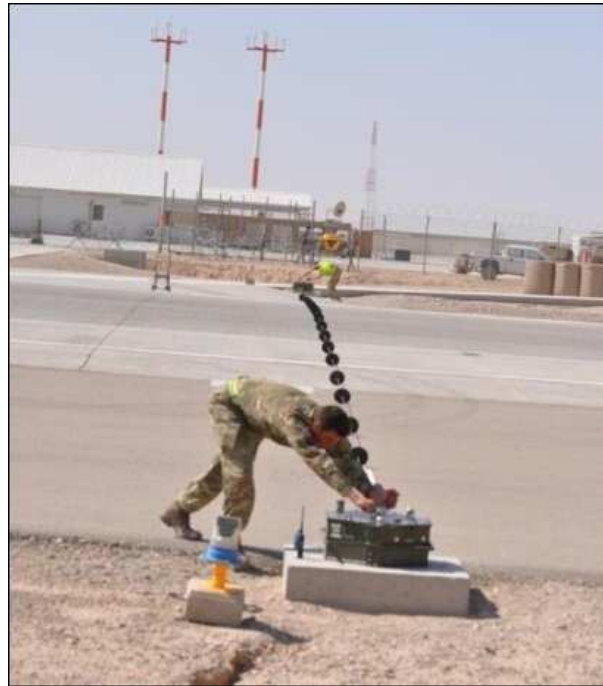
Fig. 2.2 Watchkeeper WK450 UAS Arrestor hook being deployed across runway. [104]
