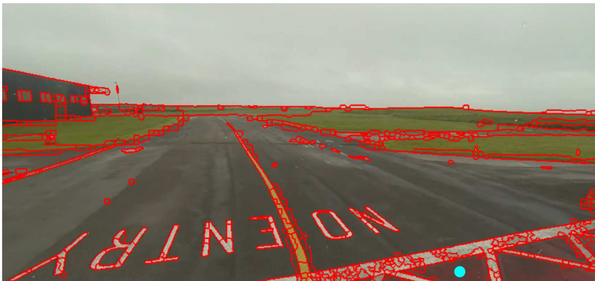
Fig. 8.8 Example image having undergone superpixel segmentation and reachability clustering.
