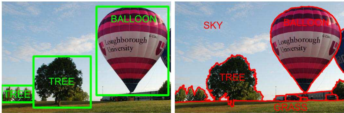
Fig. 4.5 Comparison of Object detection and Semantic Segmentation results
