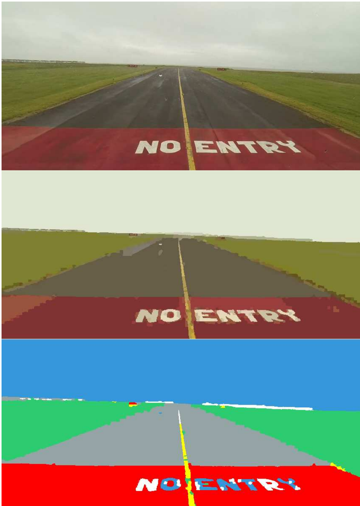
Fig. 7.12 Example of an image progressing through colour-only classification. The top-most image shows the original 24-Bit colour representation. The middle image shows the Discretised HSV colour representation, with only 2161 colours. The bottom image shows the trained Bayesian network output, using only colour classification.
