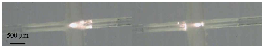
Figure 36. (Left) Light transmission from 105 \mu\text{m} fibre to 50 \mu\text{m} fibre (Right) 50 \mu\text{m} to 105 \mu\text{m} .
