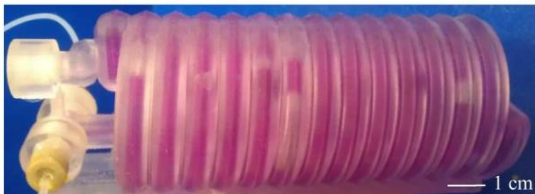
Figure 16. SL coil reactor with split and recombine mixer. Figure reproduced from reference. 77
