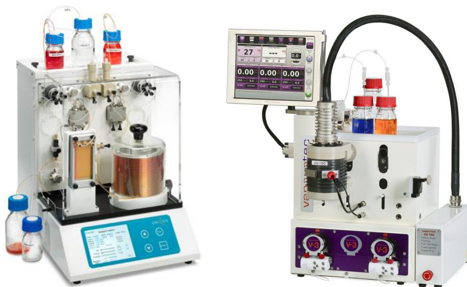
Figure 7. (Left) Uniqsis Flowsyn Figure reproduced from reference. 54 (Right) Vapourtec E series with photochemistry reactor. Figure reproduced from reference. 55
