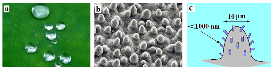
Figure 1 Lotus effect. a , Lotus leaf and beads. b , SEM image of micropapillae presented the surface of lotus leaf. Reproduced from [4] with permission from Springer. c , Nano- and
