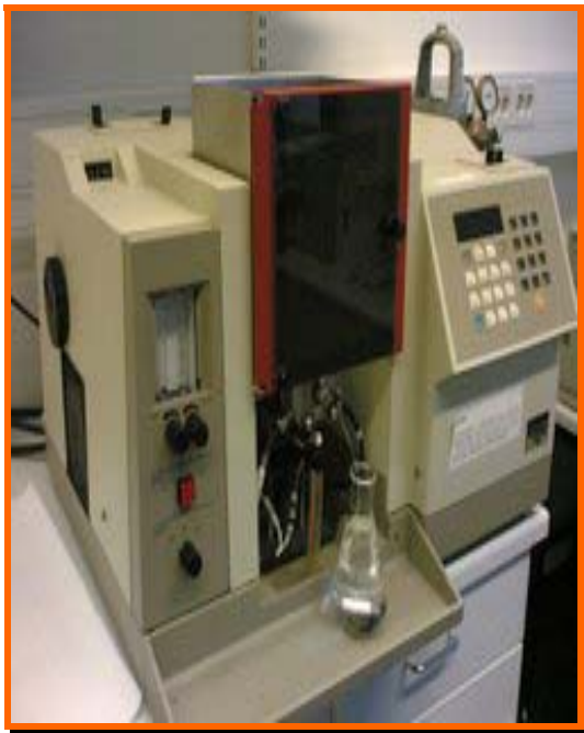
Fig. 4. Estimation of arsenic by atomic Absorption Spectrophotomete (AAS) and biochemical parameters by using Spectrophotometer (single beam).
