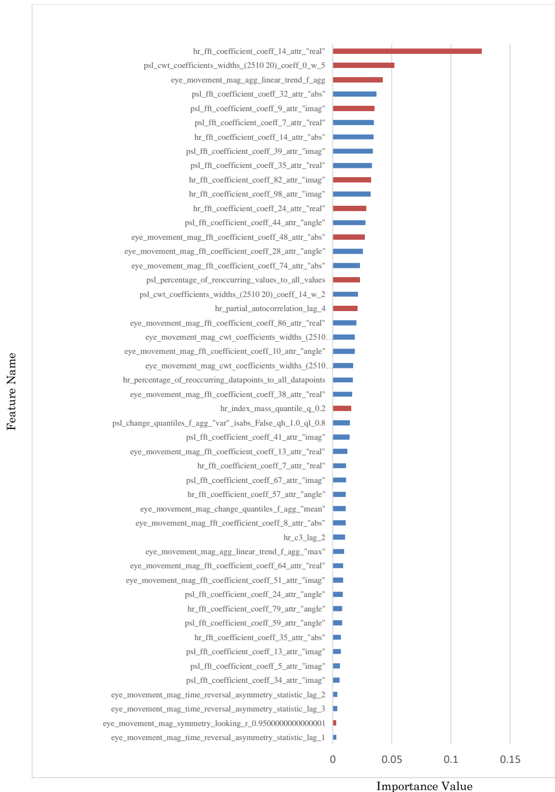
Figure 23: List of features passed to the response time regression model. Features are ranked by the random forest information gain values. Features highlighted in orange formed a subset that had the highest information gain with the least collinearity; making the best combination of features for an ML predictor.
