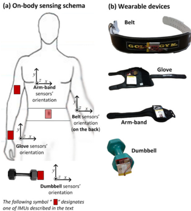
Figure 1-9 Weight lifting with sensorised weights and wearable IMUs. [61]
