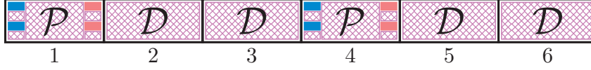
Fig. 3.30: Pilot \mathcal{P} and data \mathcal{D} blocks over B = 6 number of GFDM blocks.
