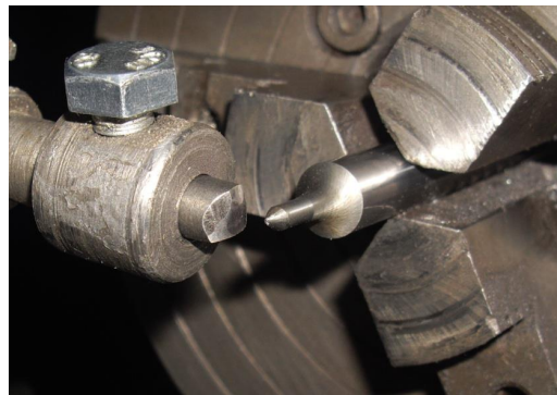
Fig. 6. Pre-installation of the mandrel for diamond knurling
