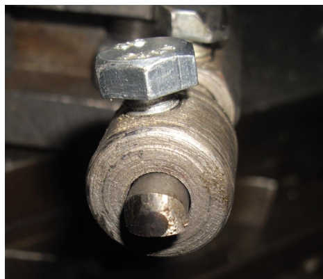
Fig. 8. The view of the working surface of the knurler made of “Hexanit-R” after 40 hours of operation
