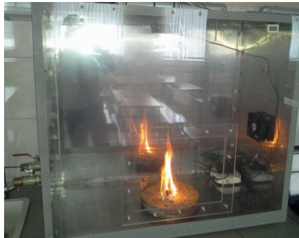
Fig. 3. Appearance of the chamber and the investigated source of material tanning
