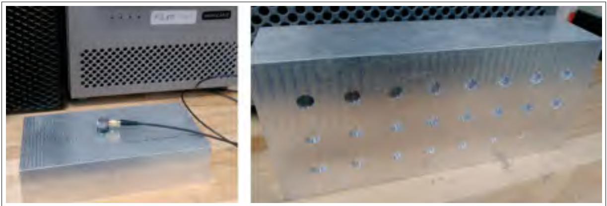
Figure 2.9 Aluminum block with different FBH depths and the Olympus V125-RM probe
