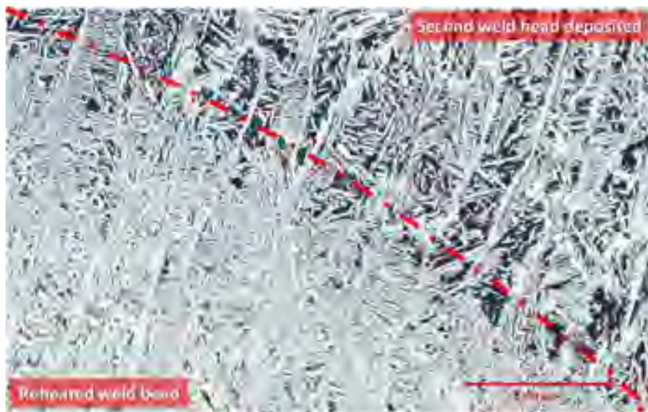
Figure 3.11 Effect of reheating in a multipass weld deposit over austenite formation
