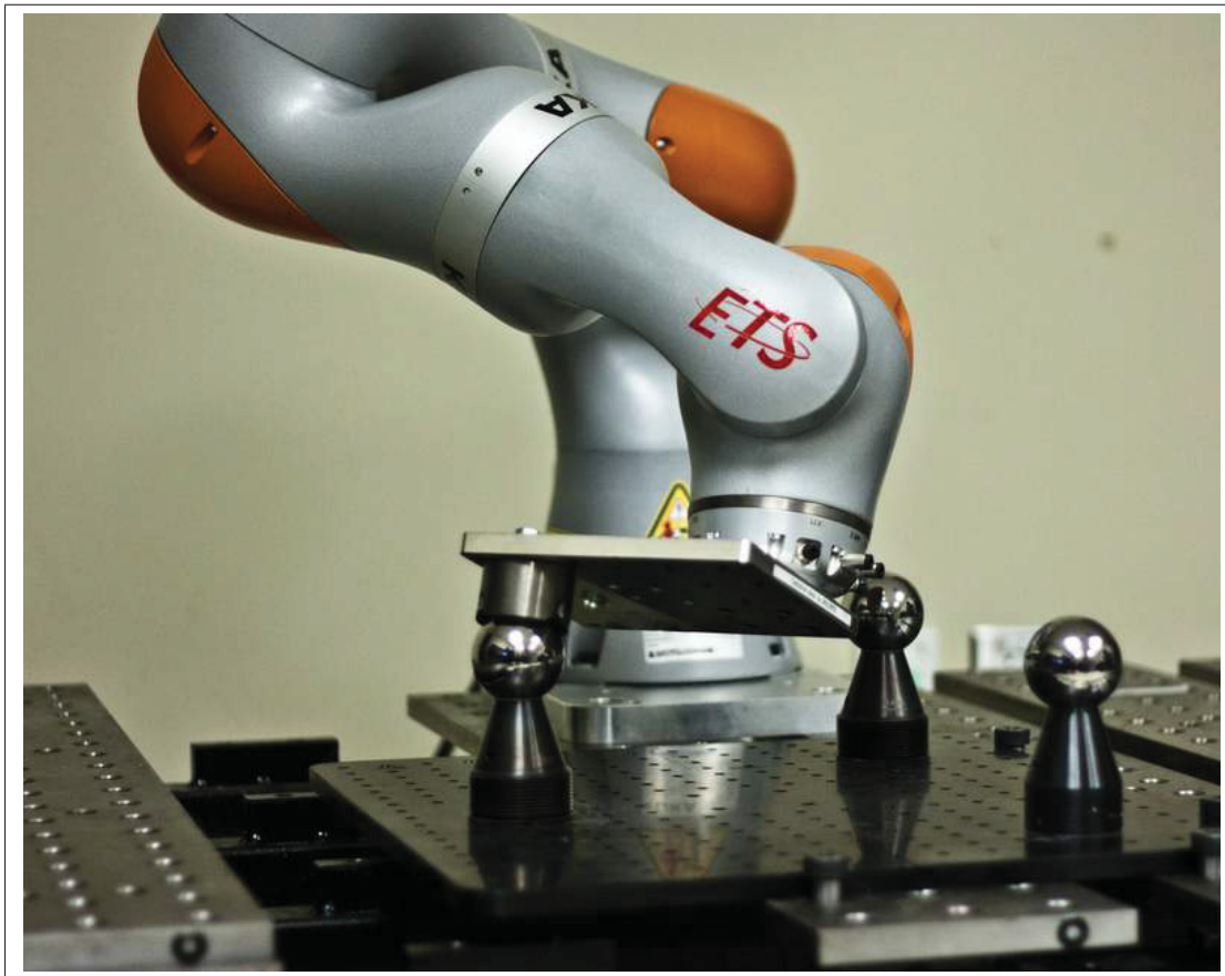
Figure 2.1 Impedance controlled calibration of a KUKA LBR iiwa 7
