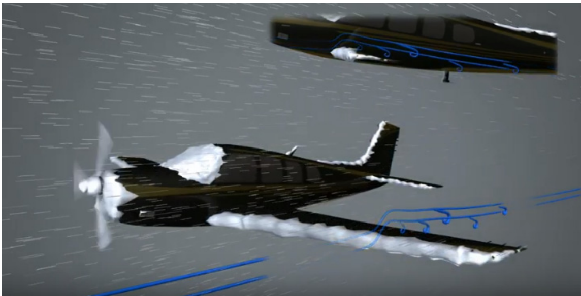
Figure 0.1 Inflight icing on the non-protected surfaces (Bremmer, 2018)
