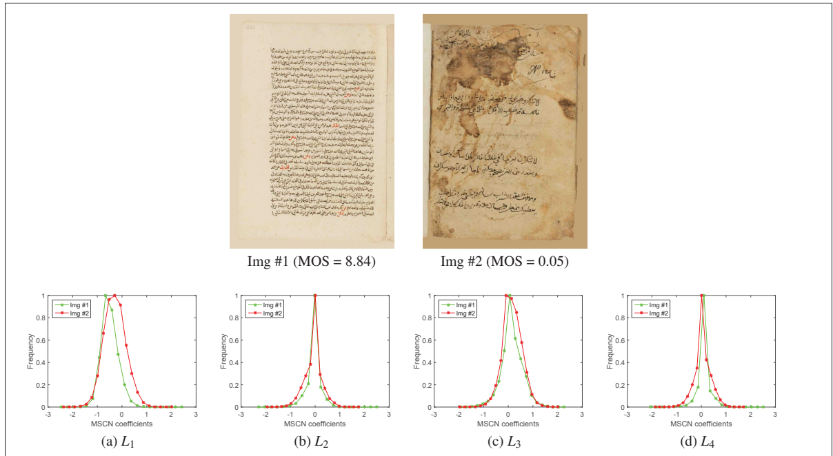
Figure 3.10 Histograms of MSCN coefficients for (a) possible text pixels, (b) possible degraded pixels far from the text, (c) possible degraded pixels close to the text, and (d) possible non-degraded background pixels.
