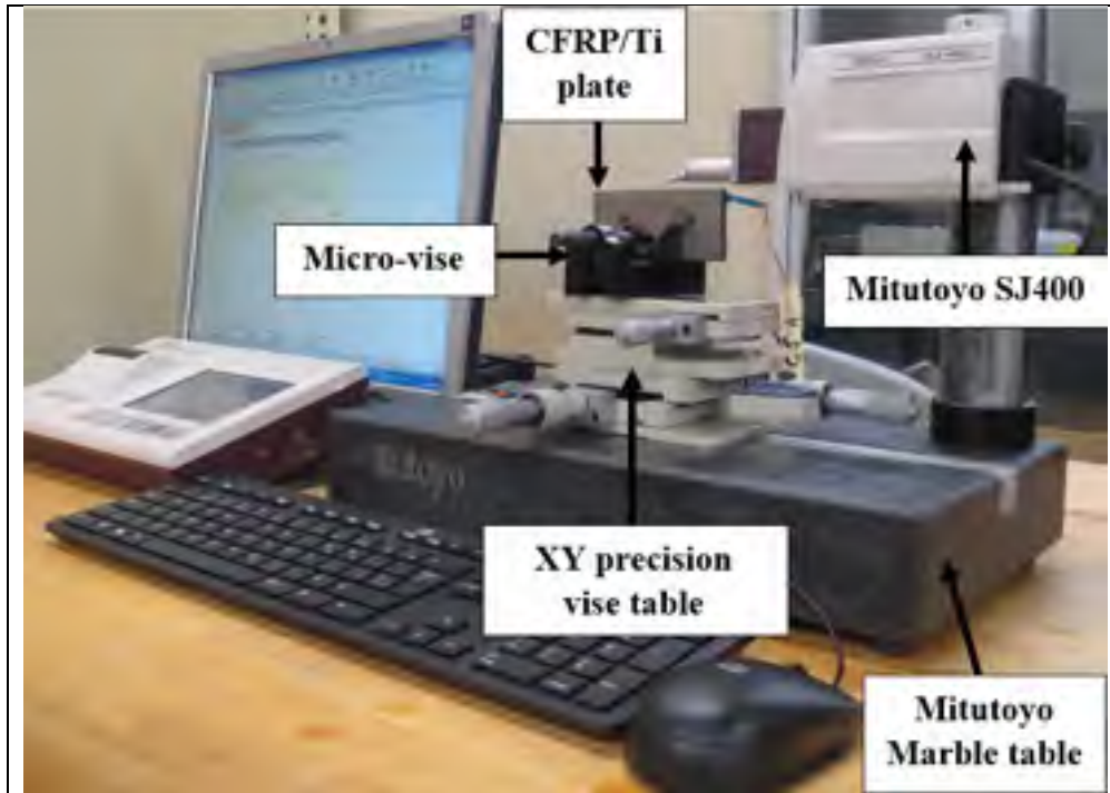
Figure 2.18 Roughness setup
