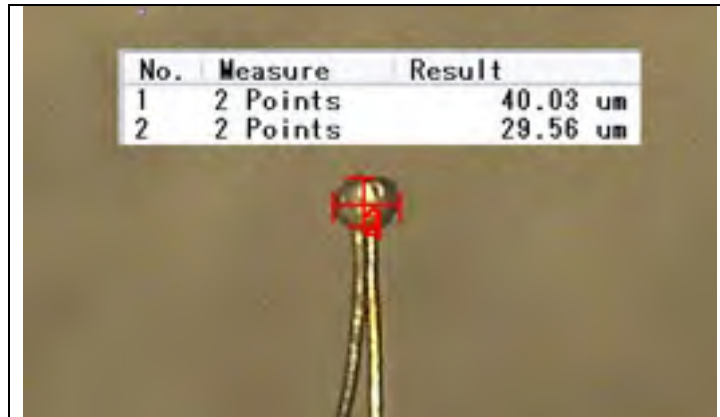
Figure 2.8 Thermocouple welding tip view
