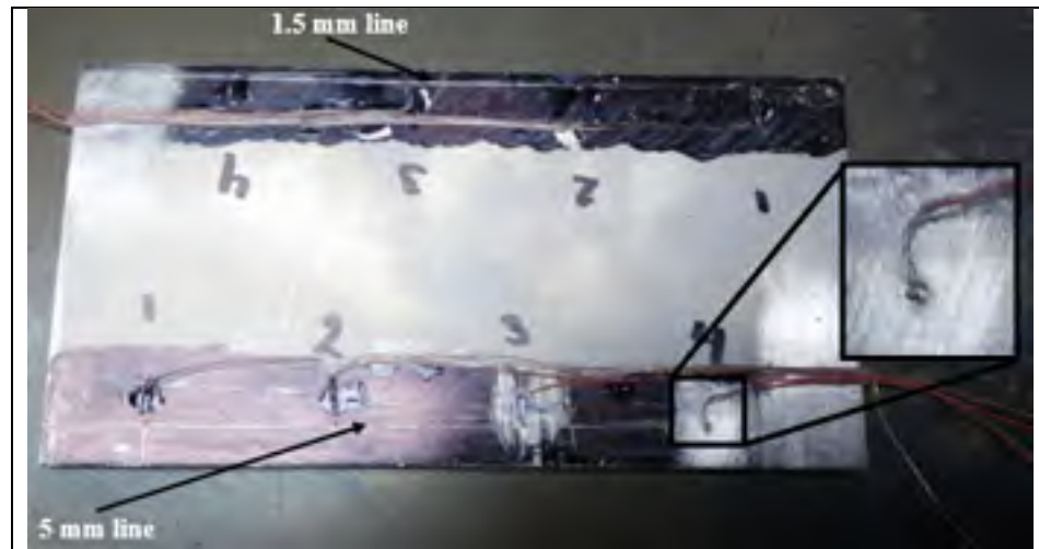
Figure 2.9 Thermocouple micro-welding sample plaque
