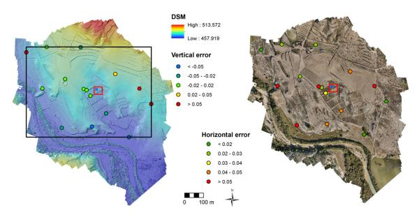
**Fig. 4** Example of the DSM (Digital Surface Model), and shaded relief with 50% transparency (left) and the orthophoto (right), produced with images from flight A1. The colored dots represent the locations of the GCPs and vertical and horizontal deviation from dGPS measurements
