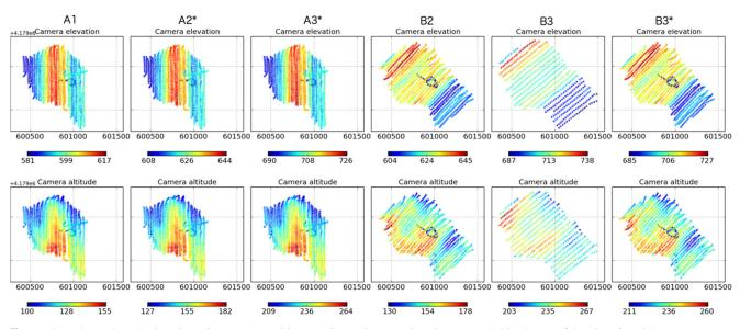
Fig. 3 The subsets show the locations (in UTM Zone 30N coordinates in [m]), elevation [m] and altitude [m] of the aircraft and the camera
