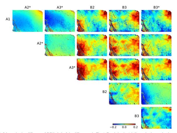
**Fig. 6** Subsets showing difference of DSMs [m] of the different flights. The labels at the left and top show which DSMs were compared. The colors from blue to red represent -0.2 to 0.2 meters difference. The location of the subset is shown by the black rectangle
