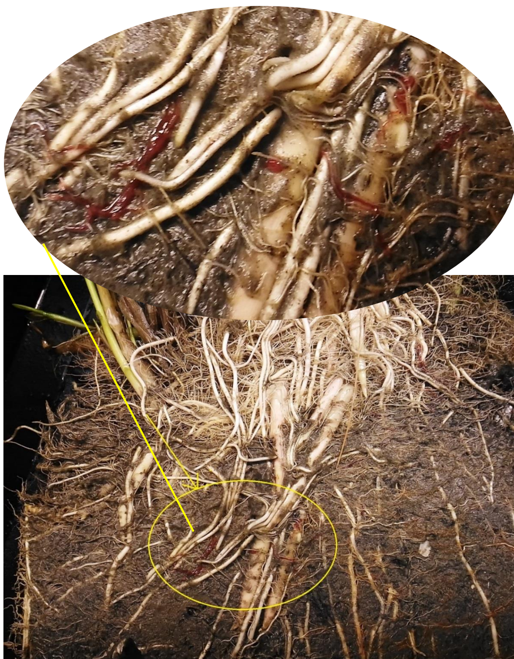
Figure 3. 5: Worms in the anode plant-MFC 3 (MS100) surviving during 190 day operation
