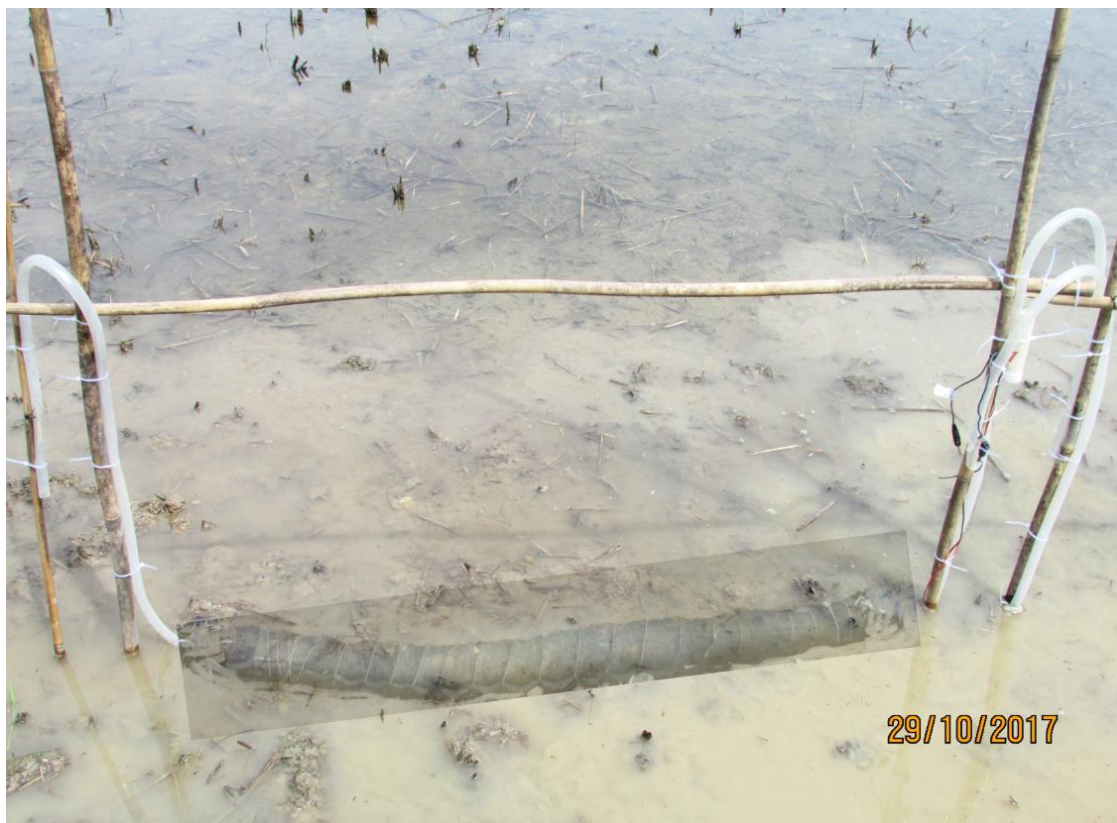
Figure 4. 3: Installed tubular Plant-MFC installation (see shaded area) just before covering the tube with paddy field soil
