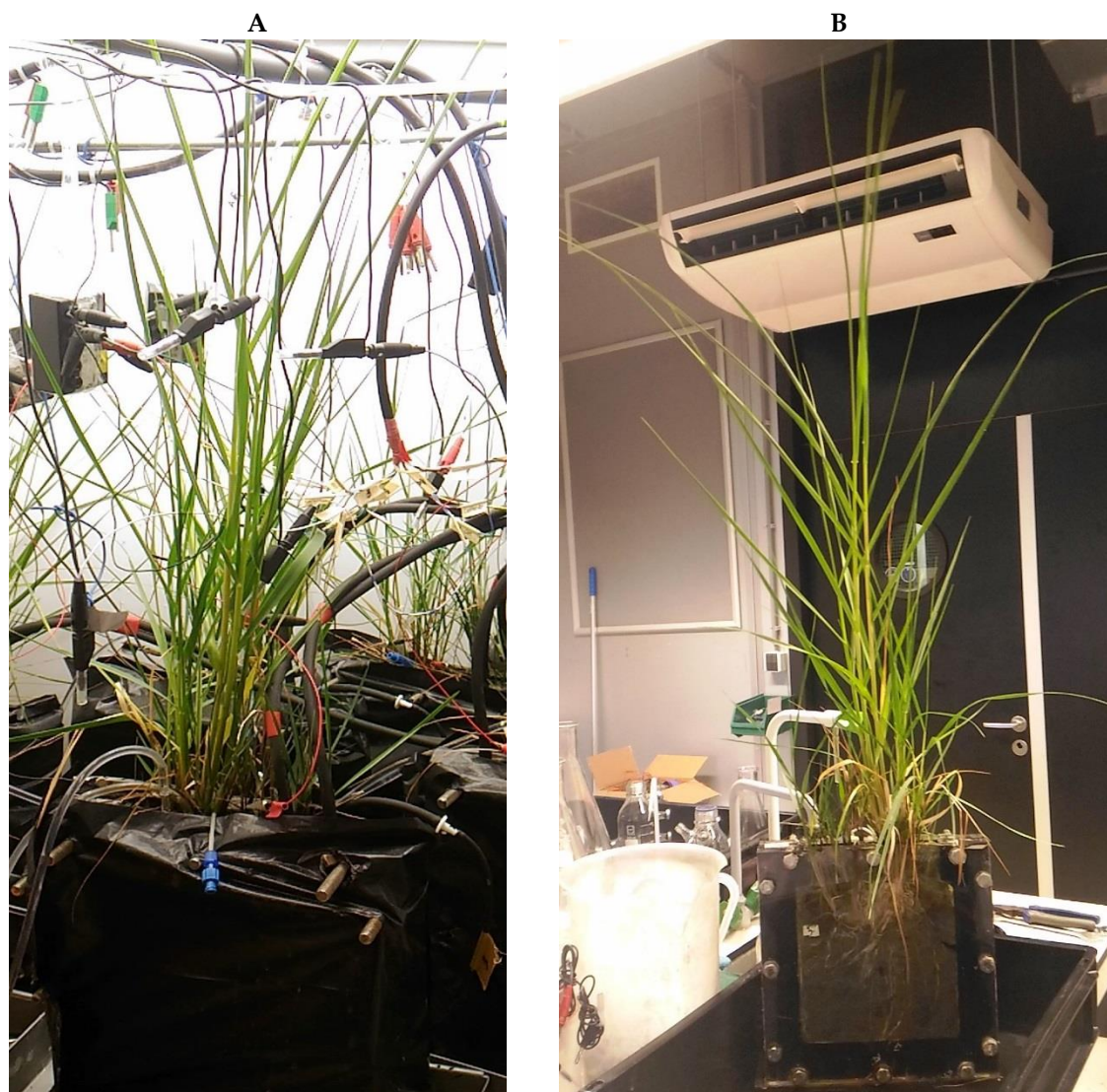
Figure 3. 1: Full-grown Spartina anglica in plant-MFC 3 (MS100); (A) inside the climate chamber and (B) at the end of the experiment
