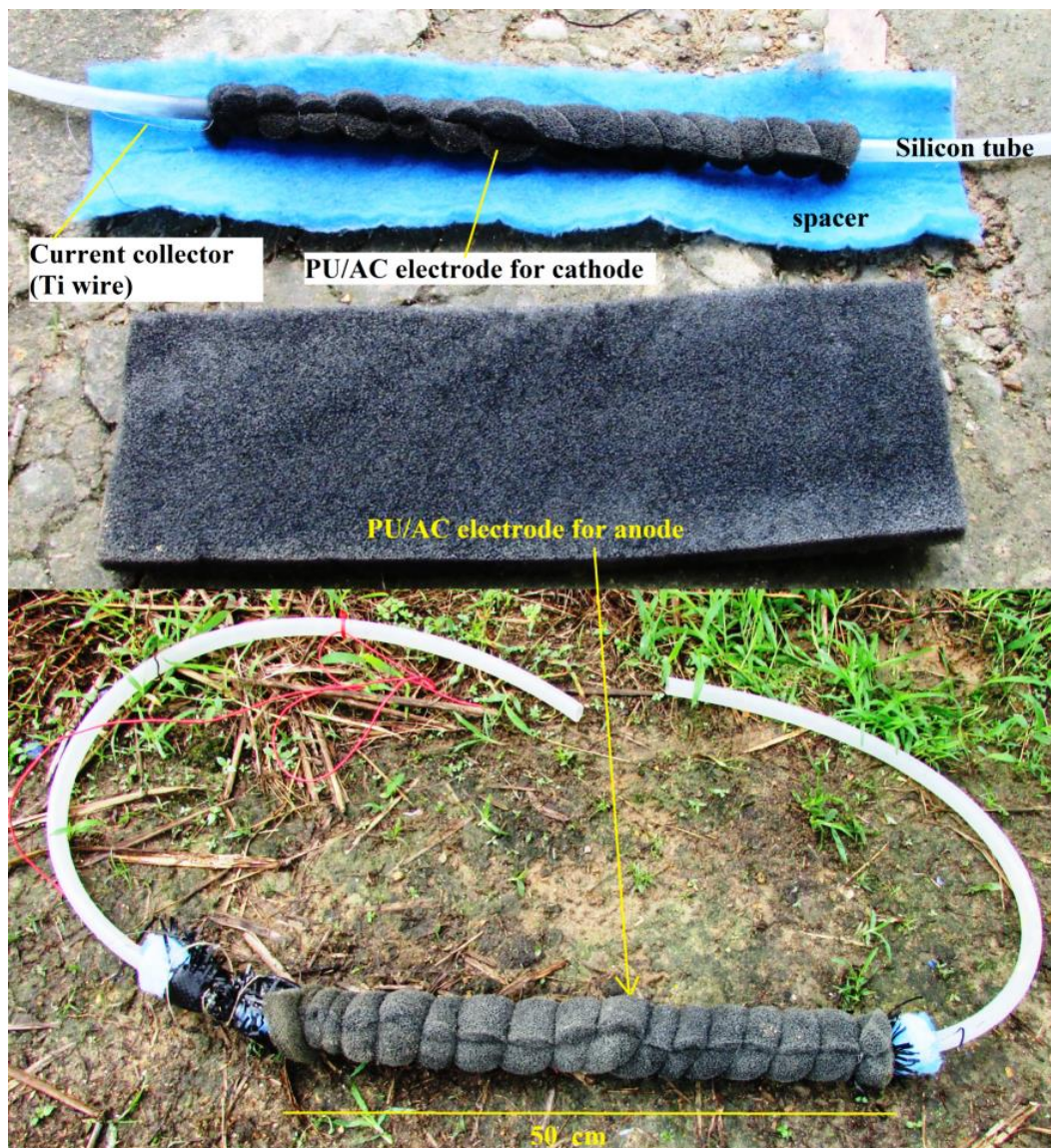
Figure 3. Materials and completely constructed tubular Plant-MFC with PU/AC electrode.
