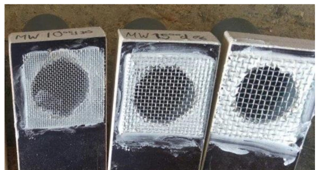
Figure 5. The ability of small hive beetle larvae to pass through three sizes of test meshes (1, 1.5, and 2.5 mm, from left to right) was determined (photo: K. Stief).
