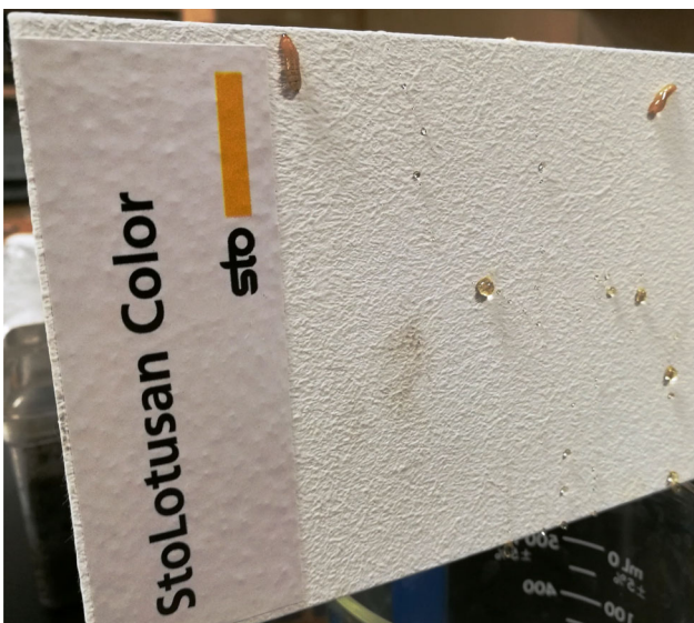
Figure 4. A small hive beetle larvae crawling up the surface of a piece of cardboard coated with StoLotusan Color™ (photo: K. Stief).
