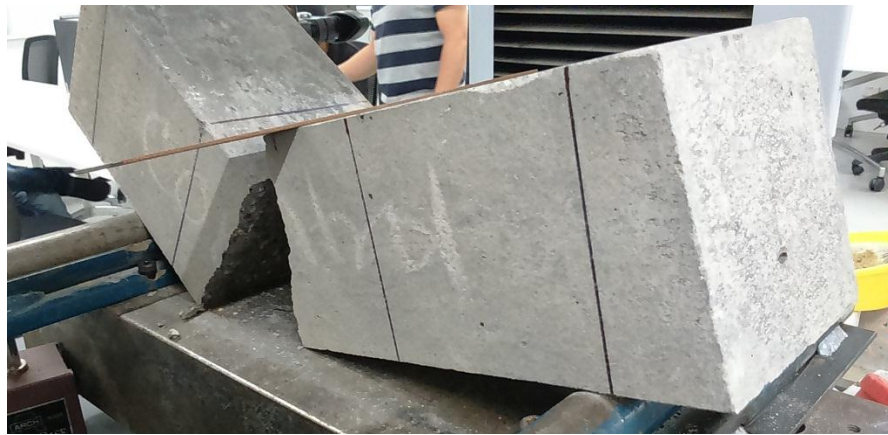
(a) Failure load – 17066.7 N
