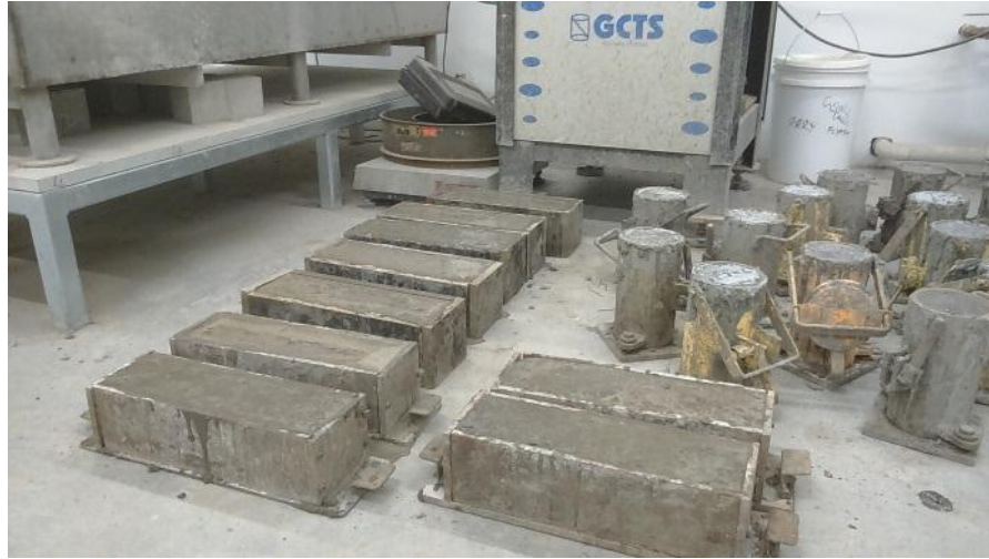
Figure 5-6: Specimens after casting
