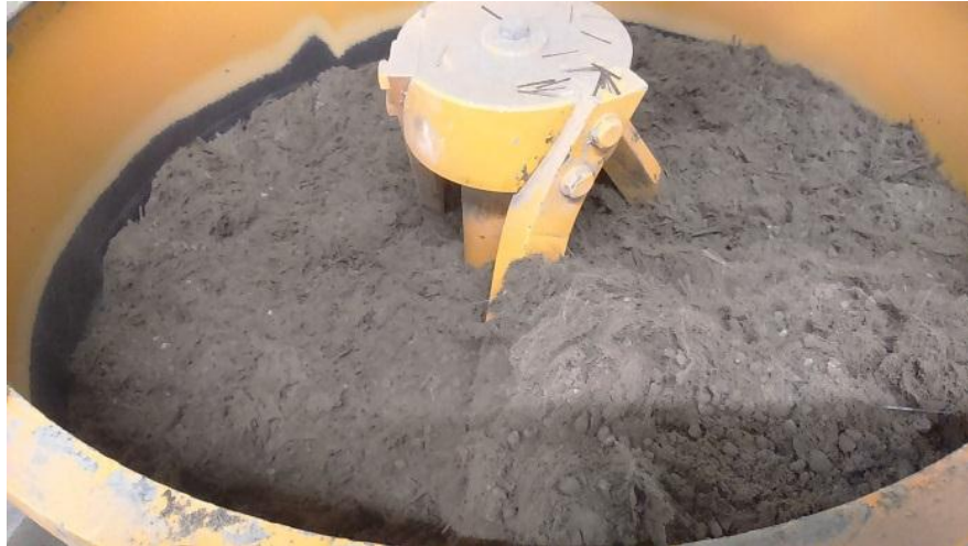
Figure 5-4: Mixing of dry materials
