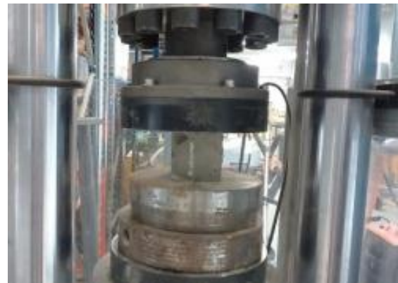
Figure 4-5: Compressive Strength test
