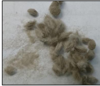
Figure 3-4: After 62 days treatment with \text{Ca}(\text{OH})_2 solution (Group B)
