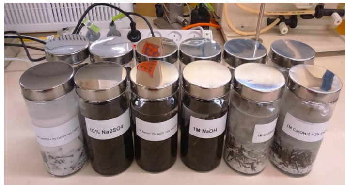
Figure 3-1: Immersion of Basalt Fibers in twelve chemical solutions
