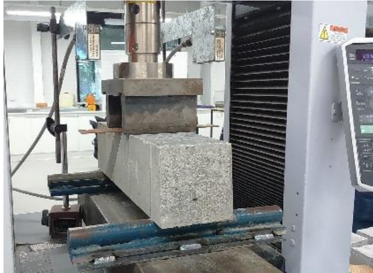
Figure 5-11: Flexural strength test
