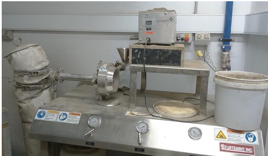
Figure 5-2: Grinding raw fly ash using micronizer
