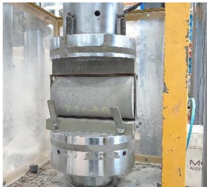
Figure 5-10: Splitting tensile strength test
