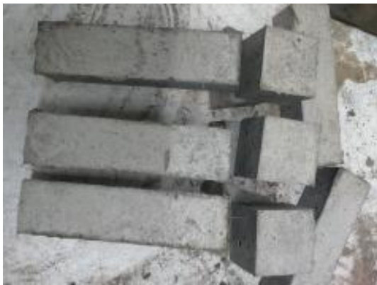
Figure 4-4: HVFA Cement mortar specimens
