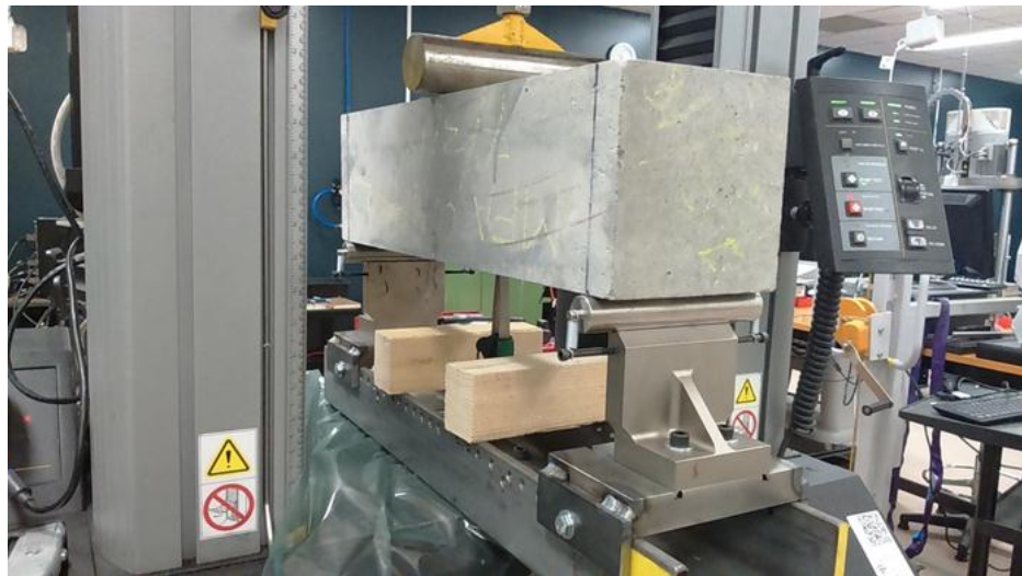
Figure 5-14: Notch beam test set up
