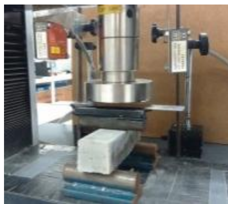
Figure 4-6: Flexural Strength test
