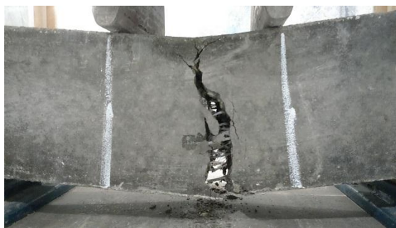
(vii) Expt. Failure crack – 26700 N
