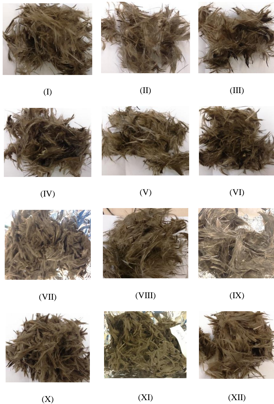
Figure 3-2: Group A basalt fiber after 62 days treatment (Table 3.4 is referred for solution Nos.)
