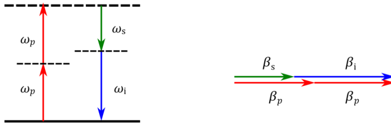
Figure 7: The energy diagram of the degenerate four-wave mixing process (left) and the collinear matching of the propagation constants (right)
