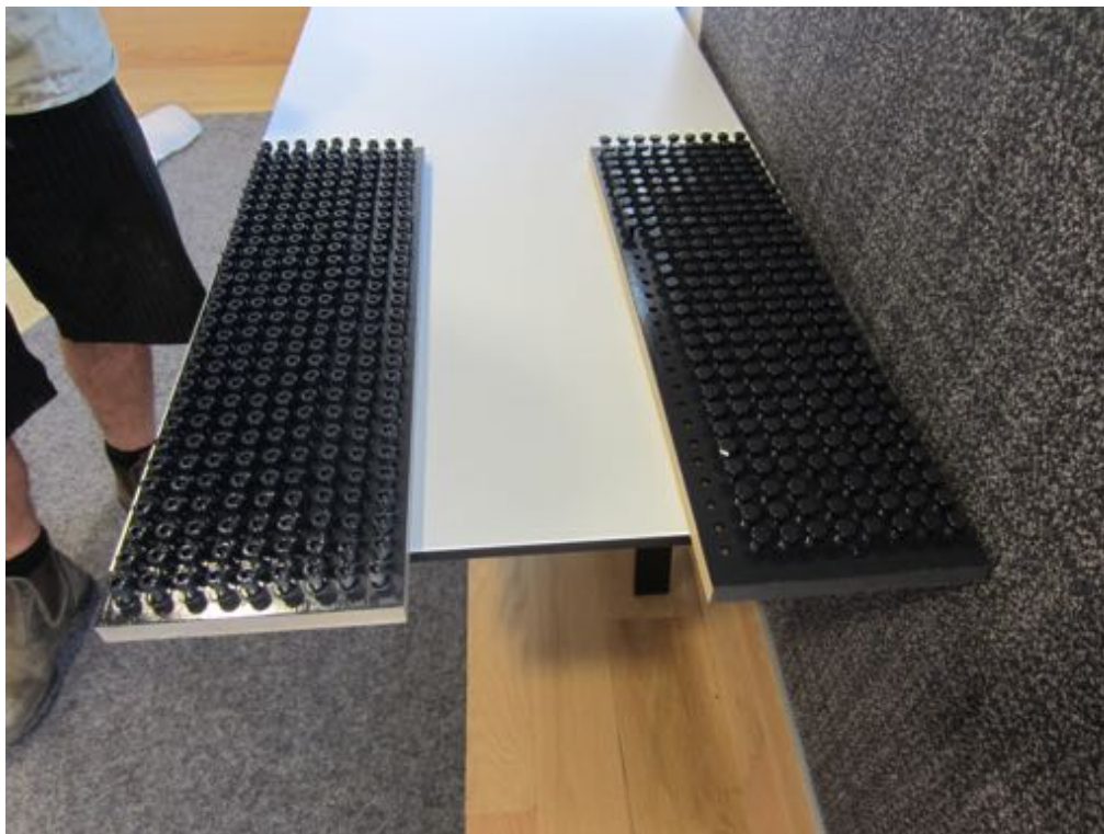
Figure 2.52 Grub screws designed to hold two-part brackets together in preparation for wall mounting. Photo – ©Simon Perry
