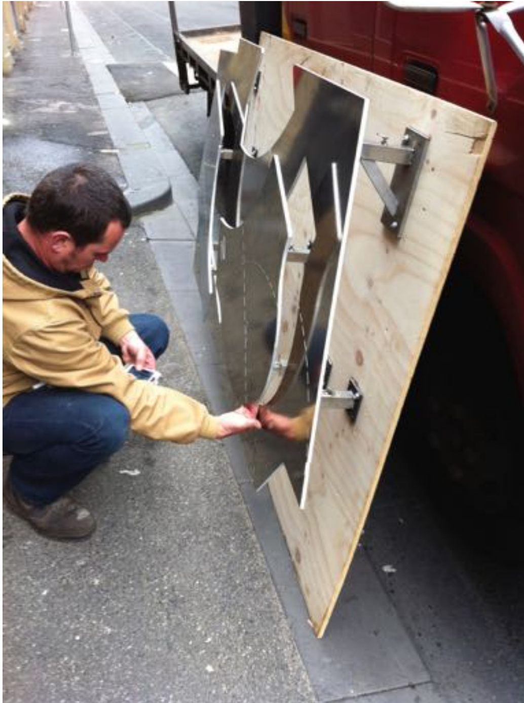
Figure 2.48 Test panels were produced to test various connection designs, scale, lighting and colours. Photo – ©Simon Perry
