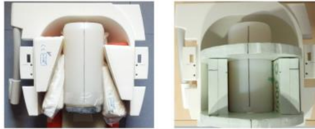
Figure S2: Manual alignment of the phantom using soft foam rubber pads (left) and more reliable alignment of the phantom using a Styrofoam holder (right).
