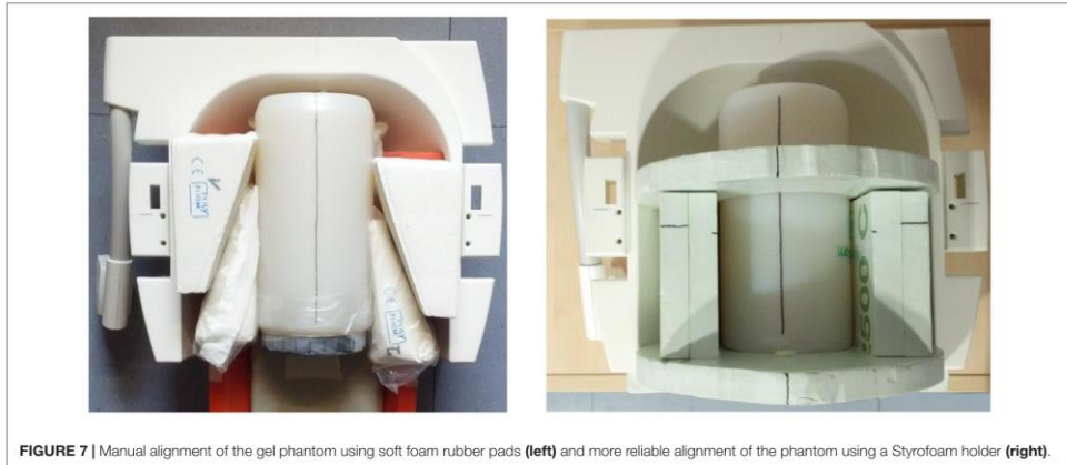
FIGURE 7 | Manual alignment of the gel phantom using soft foam rubber pads (left) and more reliable alignment of the phantom using a Styrofoam holder (right).
